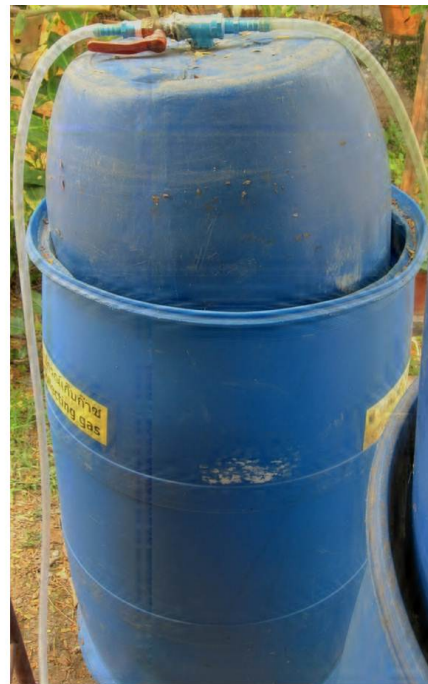
Figure 2. Bioreactor with some biogas
